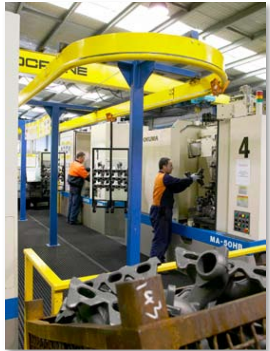
Continuous flow machining of engine manifolds at Frontline
